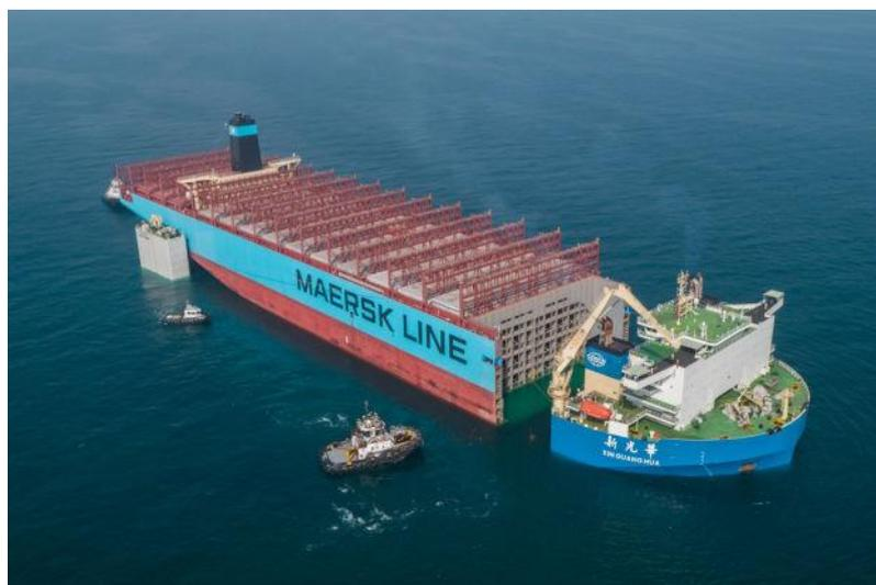
*The undamaged portion of the Maersk Honam was loaded onto a special cargo transporter and ferried to South Korea, where it will be rebuilt. PHOTO: MAERSK LINE*
