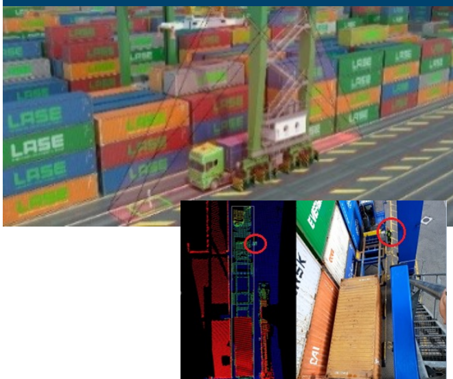
Fig 28: 3D-Point Cloud and real picture of the area (subject beside the truck in red circle)
