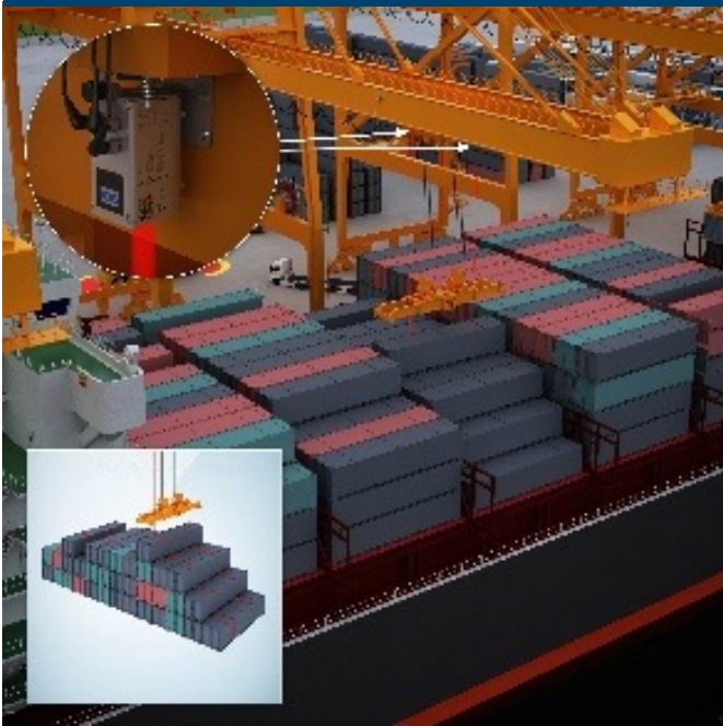
Fig 13: 1D – Laser scanner vessel profile
