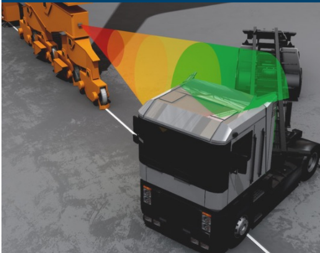
Fig 6: Radar measurement from crane-to-crane and pathway
