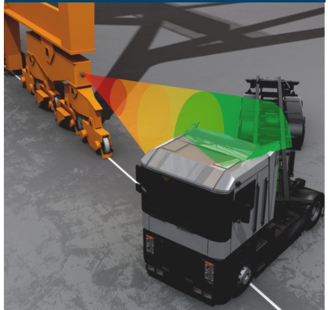
Fig 26: Radar measurement from crane-to-crane and pathway
