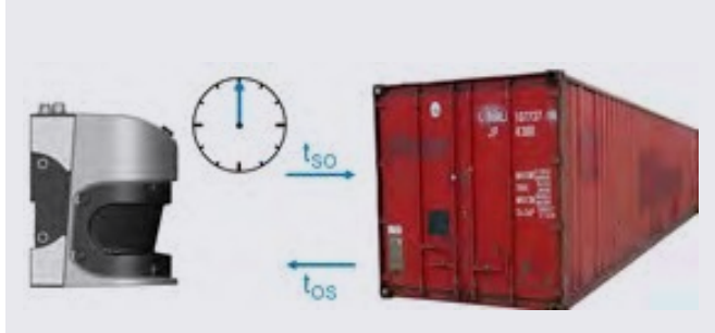
Fig 45: 2D-Laser measurement principle time-of-flight
