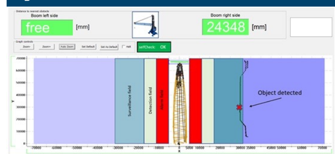
Fig 37: Visualization of the boom and the collision areas
