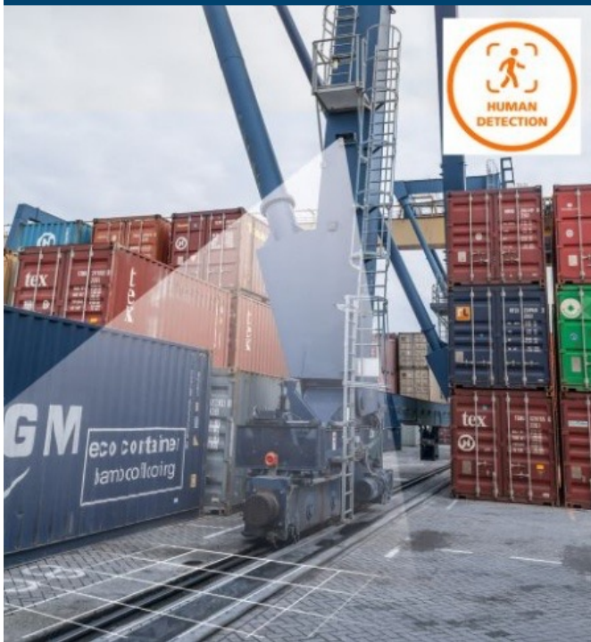
Fig 25: 3D-TOF looking down on the travel path
