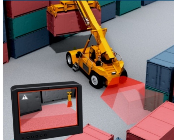
Fig 41: Reach stacker collision prevention system based on camera technology
