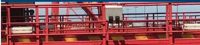
Fig 17: 2 x 3D-TOF (black boxes in the middle)
