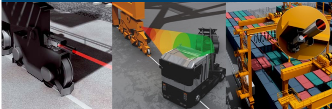
Fig 21: 1D- Laser measurement or radar at bogie level, 1D-Laser on the portal girder
