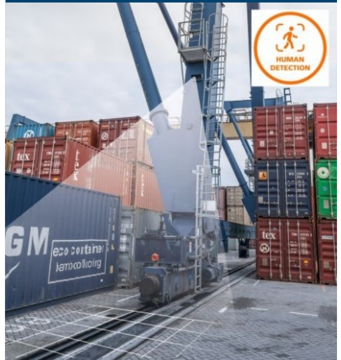
Fig 5: 3D-TOF looking down on the travel path
