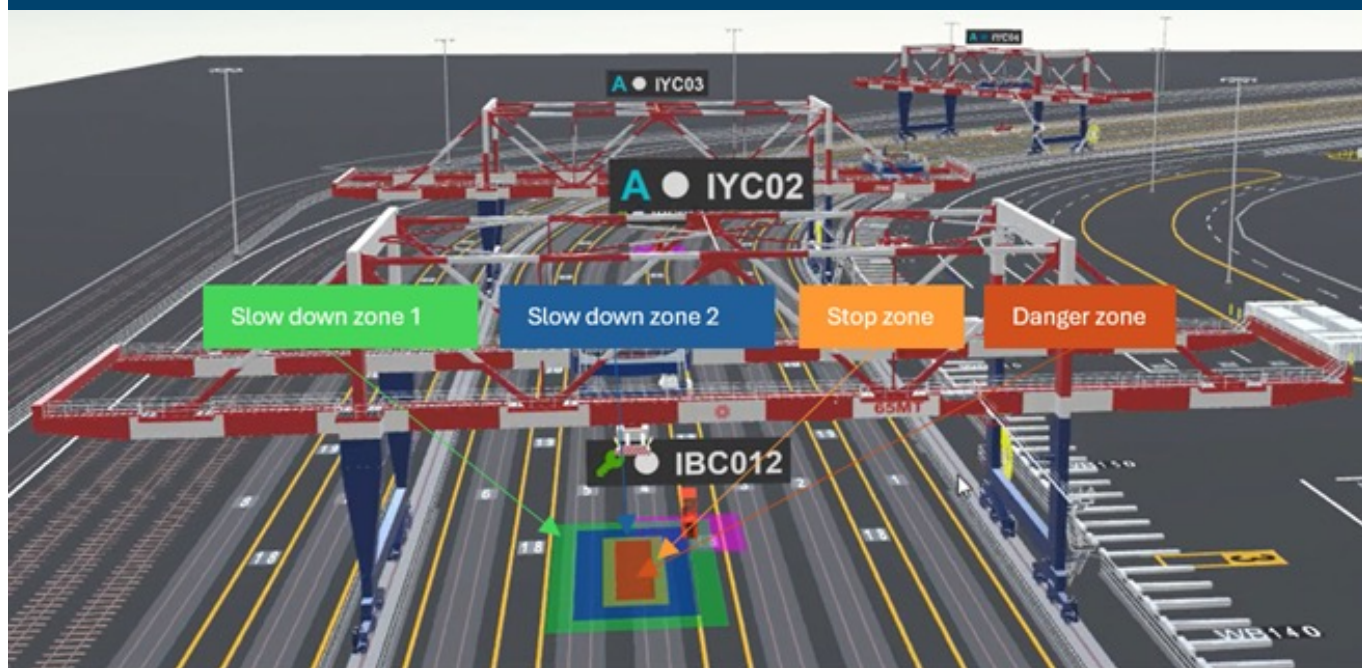
Fig 43: Multi-layered exclusion zones
