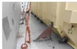
13. General view of the sea fastening along the port side of the transformer; starboard side was similarly secured with stoppers and cargo chains for uplift
