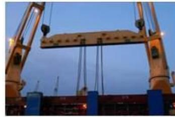
3. Ship's tandem lifting gear prepared for the loading of the transformer
