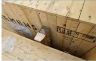
18. Where necessary, gaps between cases are choked off
