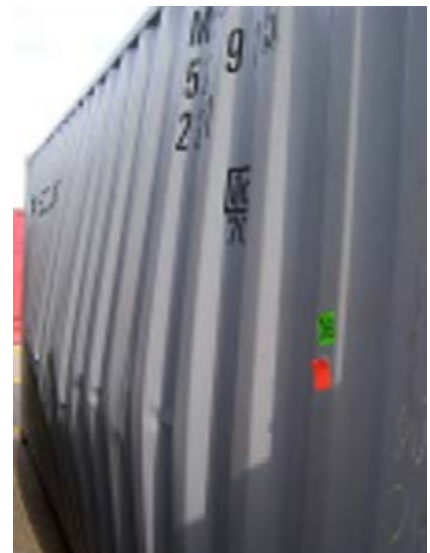
Picture 8 – Damaged side wall following road transport (Image Courtesy ETS Consulting)
