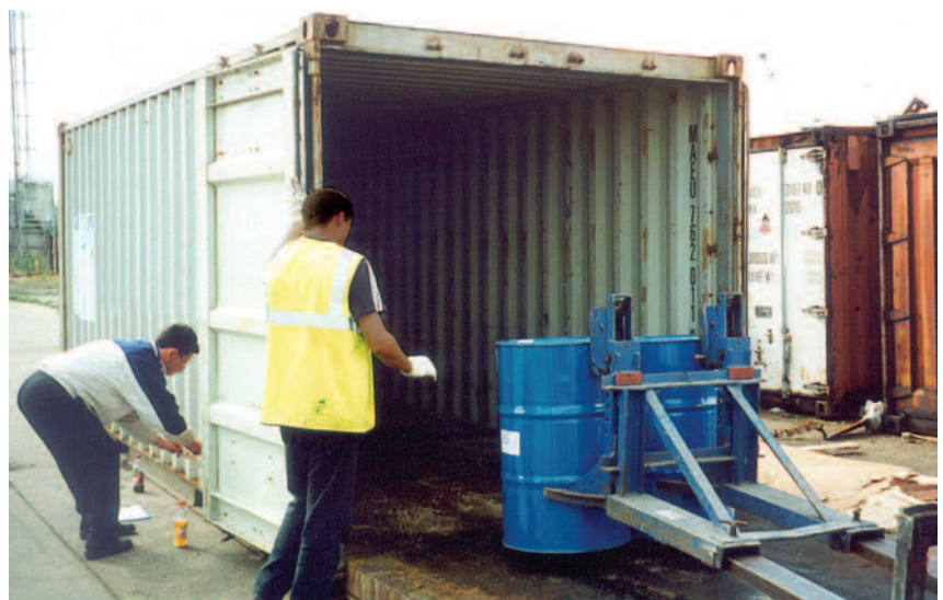
Drums being packed with drum clamps
