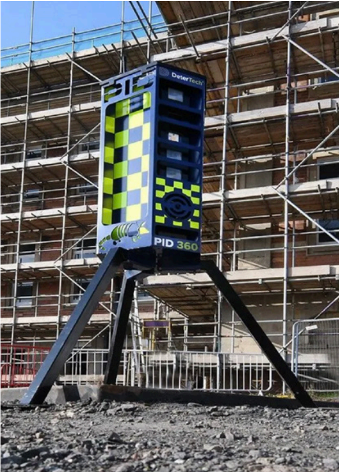
PID 360 uses motion detection and thermal imaging to identify potential threats, triggering instant alerts.
