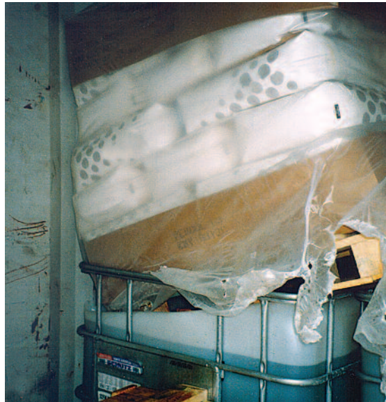
The inner plastic receptacle of this IBC has partly collapsed under the weight of a pallet that has broken through the top section of the IBC's protective metal frame
