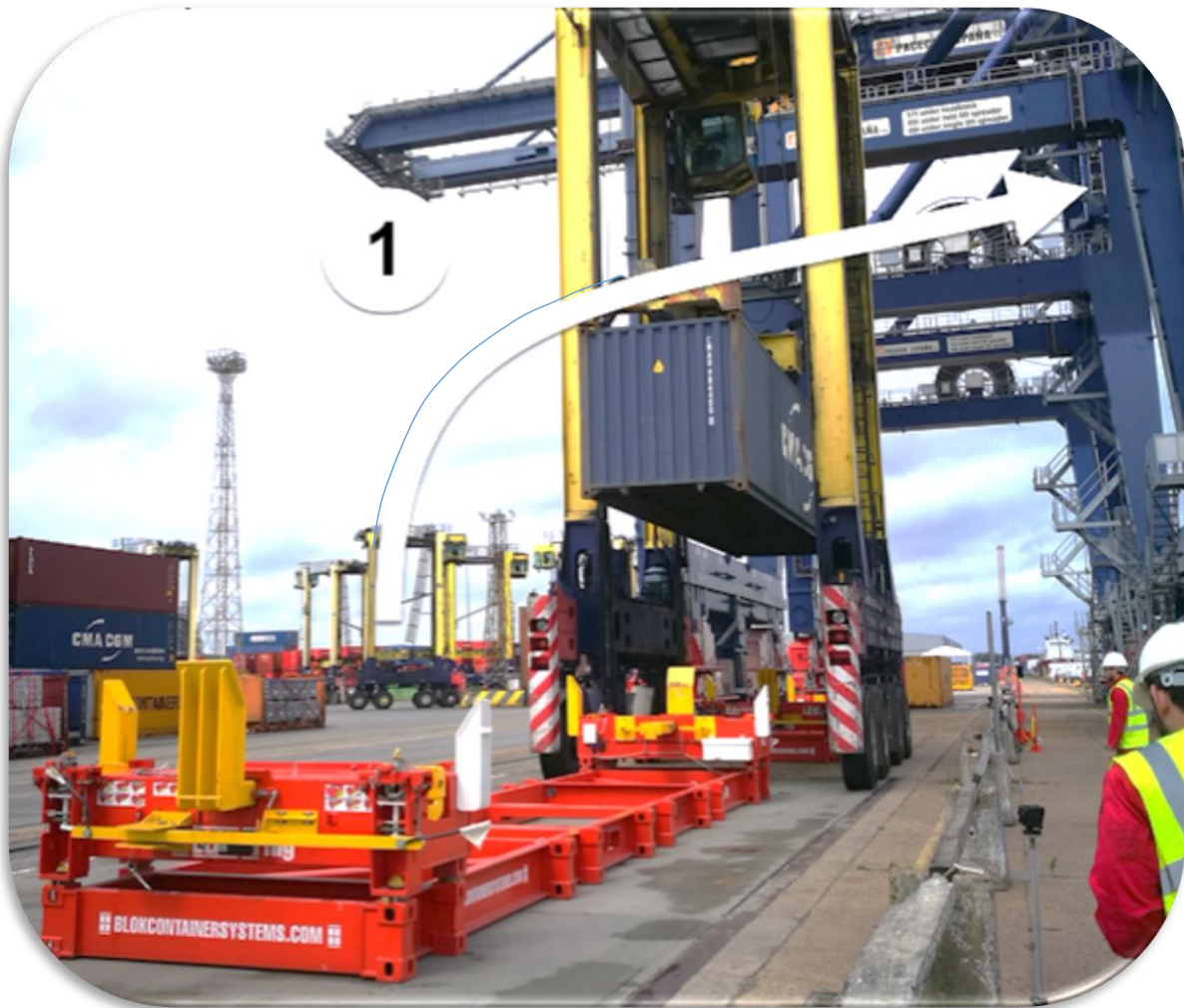
Improved process 1 x crane step = extra safety + 90 seconds cycle time
