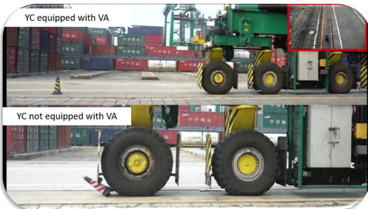
Comparison between a yard crane (YC) equipped with Video Analytics (VA) and one without (bottom)
