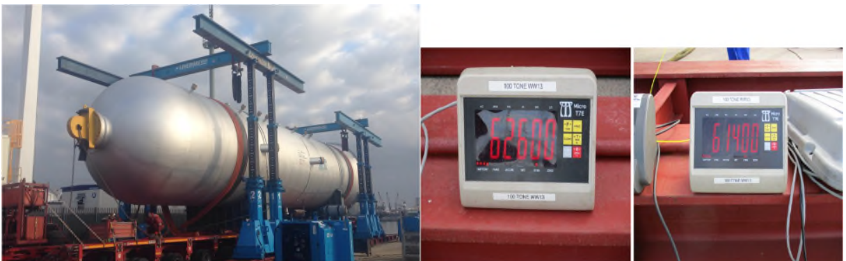
Appendix 9: Reactor prepared for reweighing via hoisting gantry. Mass of one side of the reactor was 124 tonnes which when doubled was 248 tonnes.
