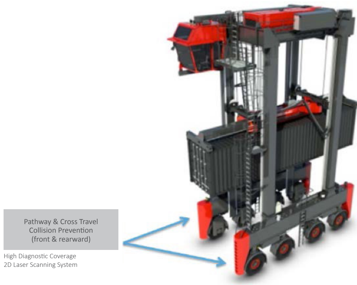
Figure: Collision Prevention Solutions at SC
