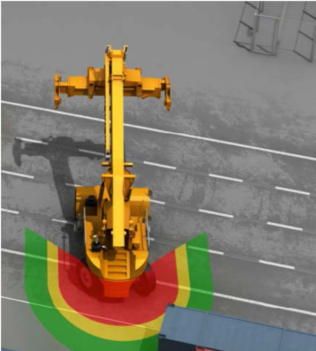
Figure: Collision Prevention Solutions at Heavy Lift Truck
