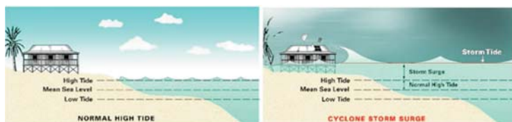
Diagram showing the impact of storm surge (Source: Commonwealth of Australia, Bureau of Meteorology)
