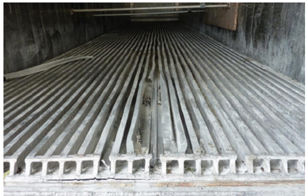
Picture 5 Badly damaged aluminium T Floor showing broken T sections, cracks to the welds which will require major and expensive repairs.
