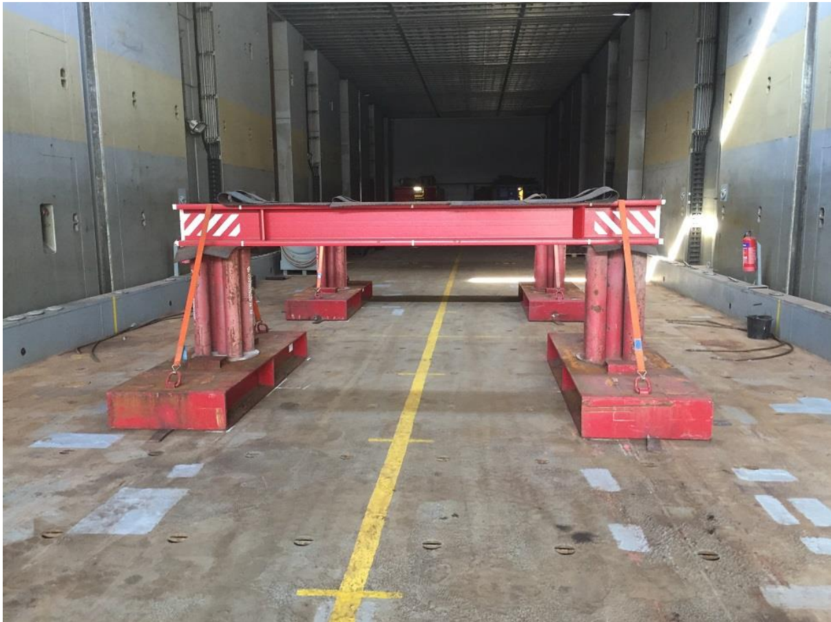
Image 2: Stool and Beam layout in the hold of the Terra Marique
