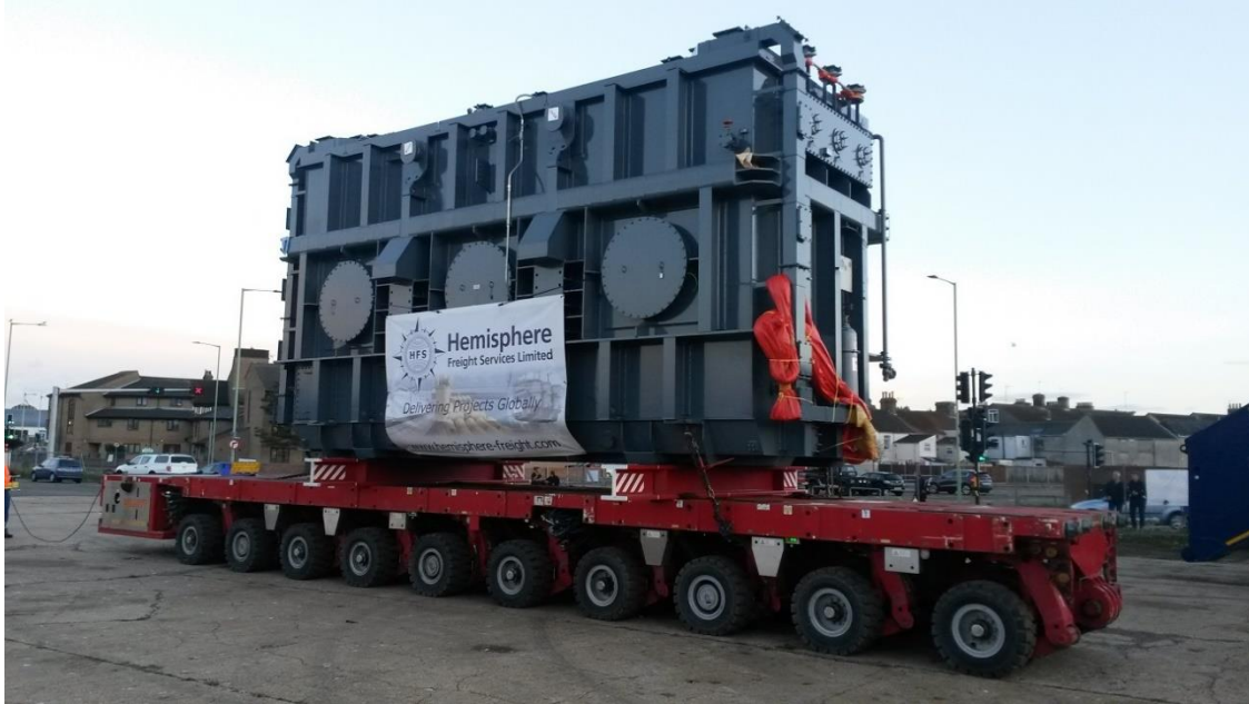
Image: Super Grid Transformer on SPMT after vessel discharge in Lowestoft
